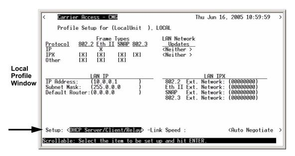
4. DHCP Mode: **<Disabled>**, **<Server>**, **<Client>** or **<Relay>**. Opens the DHCP Setup window for the following:
